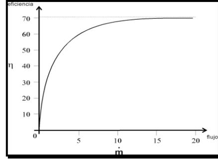
Figure 4.- Efficiency as a function of mass flow rate.
