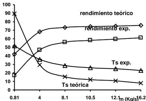
Figure 7. Output air temperature  $T_s$  and  $\eta$  as function  $\dot{m}$
