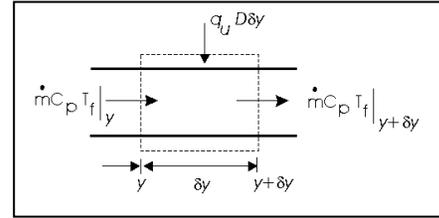
Figure 2.- Heat balance on element along flow direction
