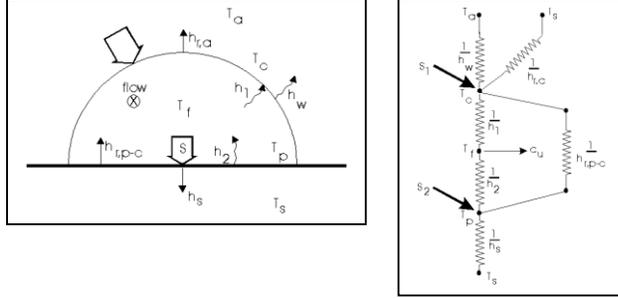
Figure 1.- Simplified model of the heat transfer in the tunnel and associated thermal network.
