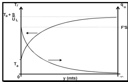
Figure 3.- Useful energy gain and outlet temperature as a function of position along the tunnel collector.
