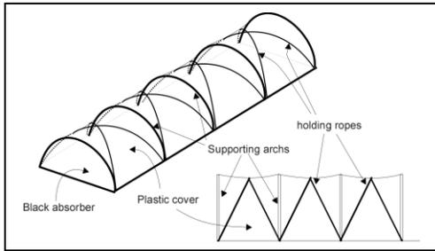
Figure 5.- Constructive details of the tunnel collector
