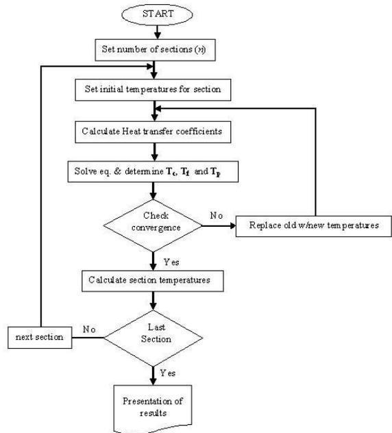
Figure 6.- Flowchart of computer program generated application.
