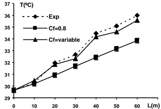
Figure 9.- Comparison of experimental and simulated air output temperatures for constant and variable friction factor.
